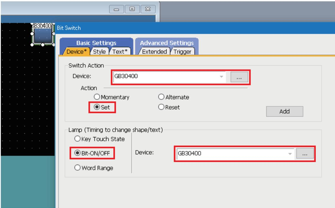
Configure the switch to open the window screen from the base screen.
