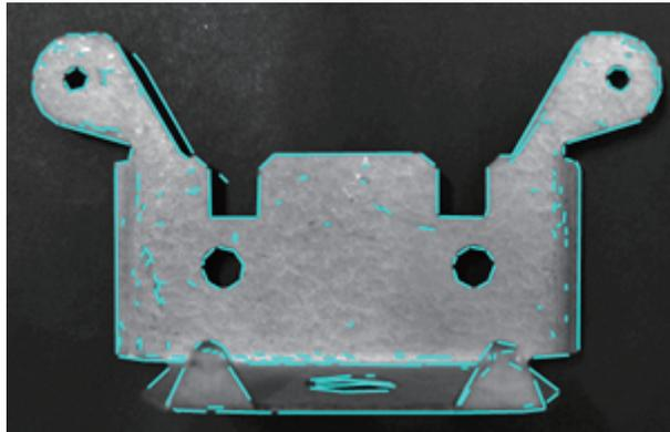
Because the edges used for calibration are detected as smart features in this case, they are used for calibration. When they are not detected, it is possible to arrange the region in which an arbitrary edge is to be detected by clearing the "Smart Features" checkbox.
