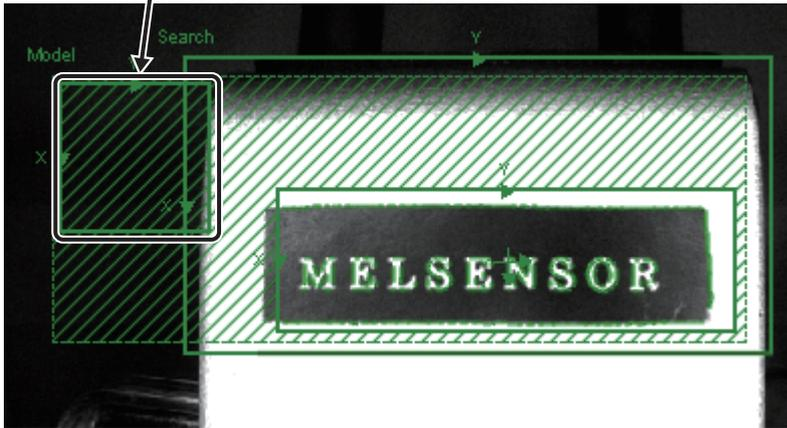
4. Configure the subtraction region so that the area outside the border does not undergo model registration.
