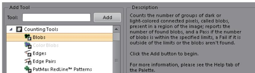
2. Arrange the inspection region so it encloses the entire region in which blobs are to be detected.
