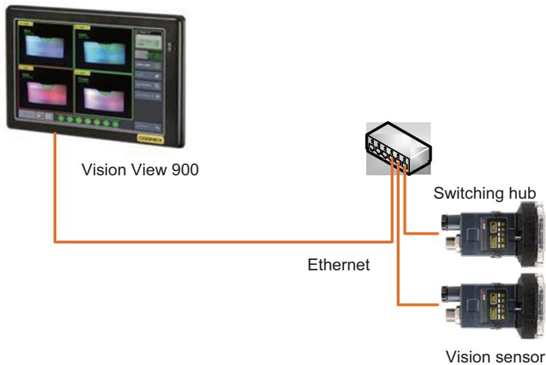
VisionView 900 is a standalone touch panel display device that can monitor the vision sensor. Monitoring is possible simply by connecting to the vision sensor. It is not necessary to create a monitoring screen.
