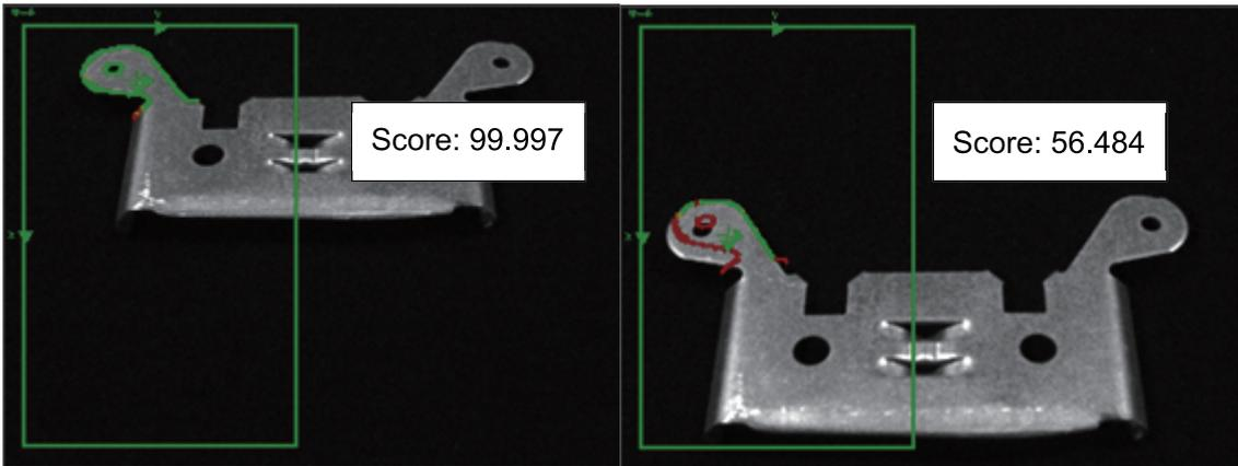
When a PatMax pattern is run while using a transformed image. (Model registration shown on the left)
