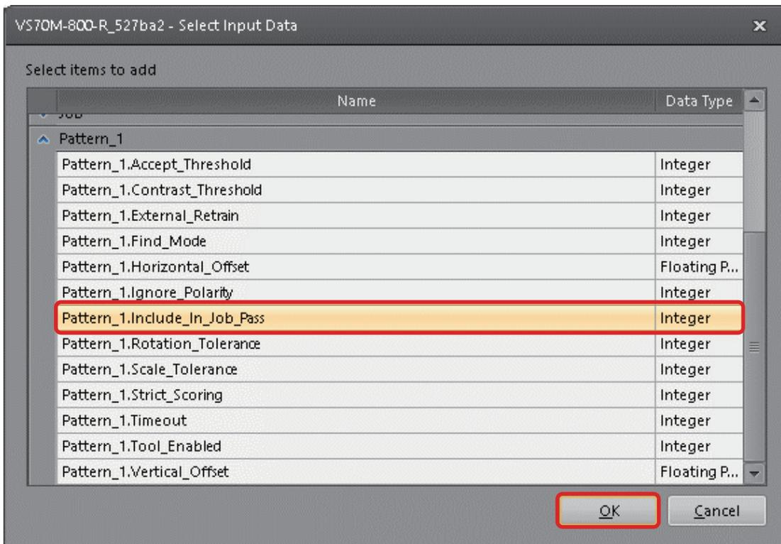
3. The parameter is added to the format input bit data.
