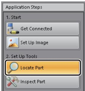
2. From Add Tool, select the appropriate location tool according to the workpiece features, tact time, and other conditions. If a location tool classification or a tool is clicked, a summary appears in the Description field to the right.
