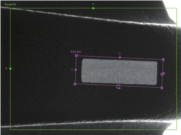
2. Add "Surface Flaw" from the "Defect Detection Tools" of Inspect Part.
