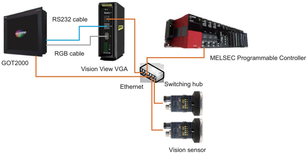
Connect the VisionView VGA and GOT using an RGB cable and RS232 cable to display the VisionView VGA image on the GOT screen.
