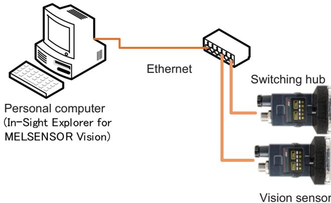
Use In-Sight Explorer for vision sensor configuration for monitoring.
