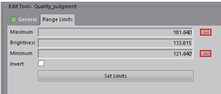
If the cursor is moved over the link icon, it is possible to check the link origin tool and content.
