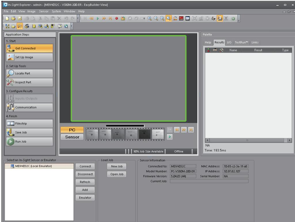
If the vision sensor to be connected does not appear in the "Select an In-Sight Sensor or Emulator" area at the bottom left, run the following procedure.
