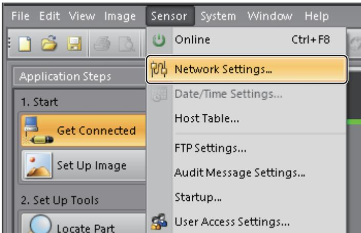
In the "Network Settings" screen, settings including IP address-related settings, validation for iQ Sensor Solution and industrial Ethernet protocol settings are available.
