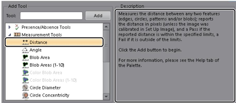
2. A smart feature is displayed in the image. Select the edge to be measured. It is possible to select the fixture position of edge tools (Presence/Absence Tools), circles (Presence/Absence Tools), and positioning tools that have already been arranged.
