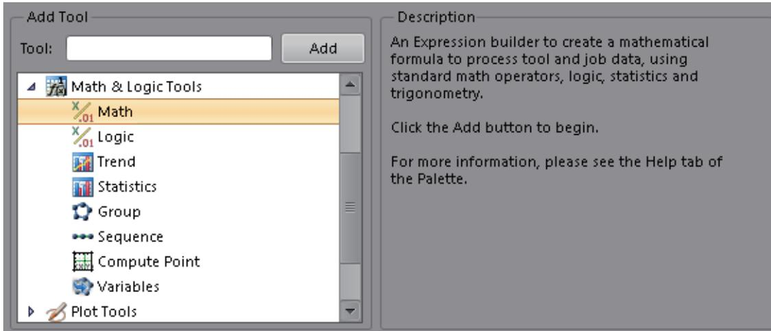
2. Insert the dimension of the Point-to-Point: Dimension tool to "Expression".
