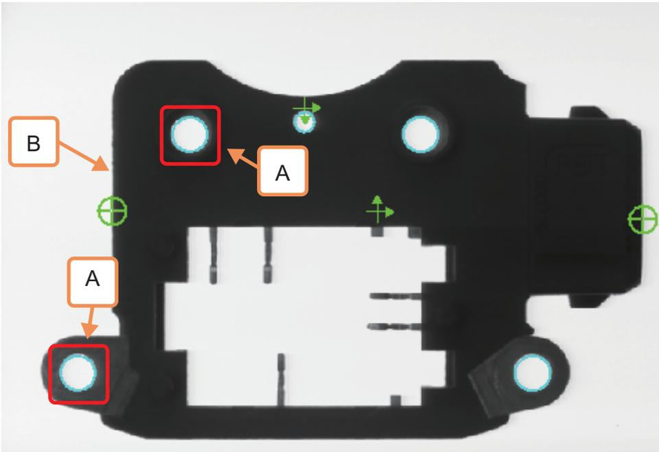
3. If configuration is complete, the display shows the distance between the two points that was measured by a line parallel with the selected edges.
