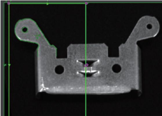
If [Transform] is used, the workpiece may not fit within the display region. In that case, set the number less than 1 to "Image Scale" in the [Settings] tab of [Transform] so that the workpiece fits in the frame.
