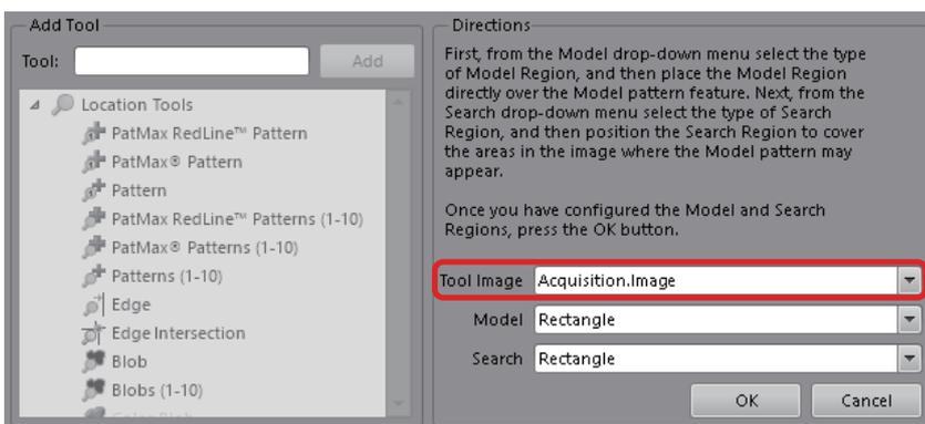
If this setting is changed to "Transform\_1.Image", it is possible to use the image that was output by Transform of the Image Filter Tools as an inspection image.
