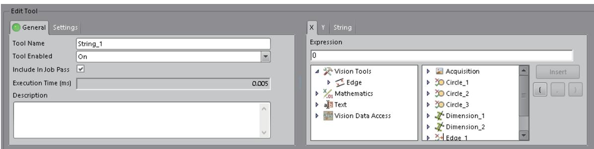
In this example, the screen displays the radius of the detected circle for Circle\_1 of the Presence/Absence Tool added automatically to detect circles when the Point-to-Point: Dimension tool was added.
