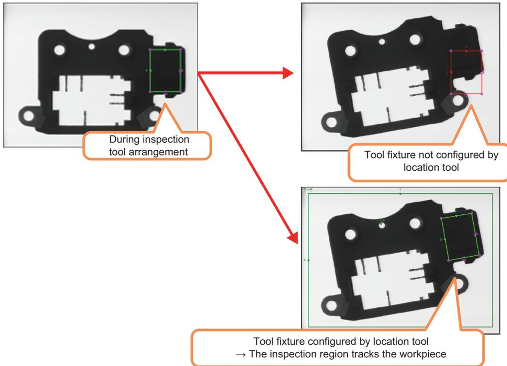
When an inspection tool is not tracking the assumed location tool, open the inspection tool and browse to the [General] tab. Using "Tool Fixture", select the location tool to be tracked.
