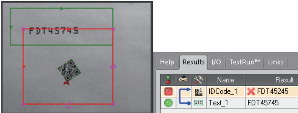
Furthermore, depending on the parameter, link icons are displayed beside linked parameters and the parameters are changed so the manual editing is not possible.
