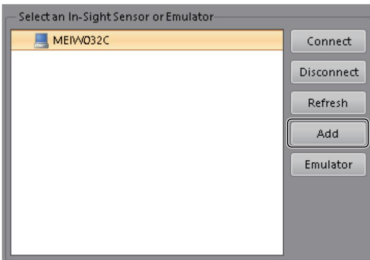
2. In the "Add Sensor/Device to Network" screen, select the vision sensor to be connected. When a personal computer cannot connect to the vision sensor, such as when the subnet of the displayed IP address is different from the subnet of the local personal computer, a warning mark is displayed on the right side of the IP address as shown in the following figure. In that case, enter an appropriate IP address.
