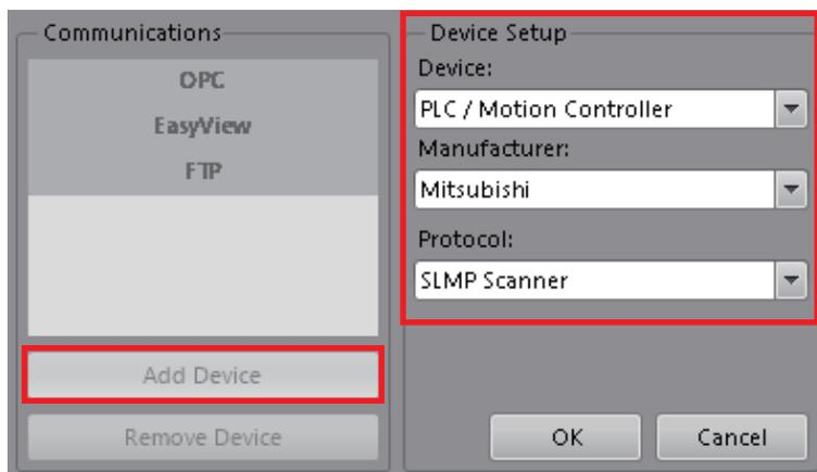
**2.** Configure the controller type, IP address, host port, and other settings to suit the communication destination.
