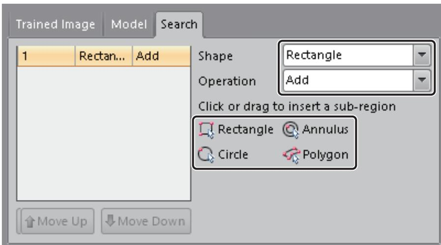
For example, when using only a border in the following model for locating part with PatMax pattern tool, add a subtraction region.
