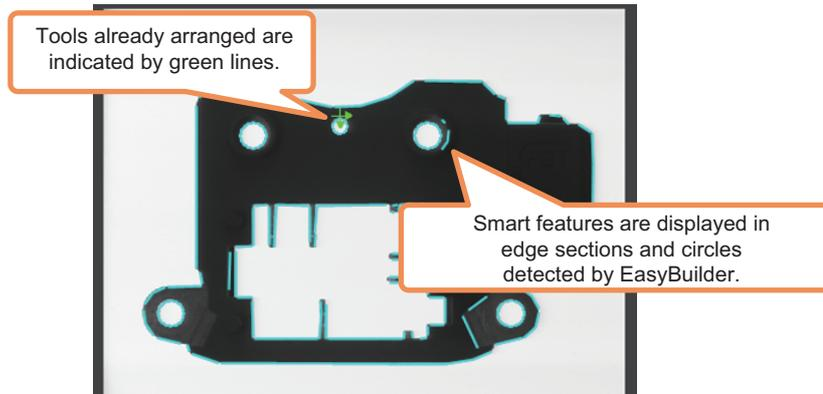
3. Click the smart features of the section to be measured in order, and then confirm the measurement locations.
