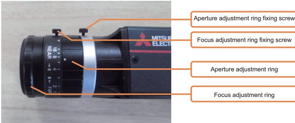
Lens aperture example (aperture may be fixed depending on the lens)
