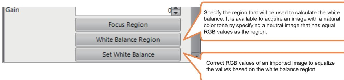
The screenshot shows the white balance settings section. It includes a Gain spinner (0) and three buttons: Focus Region, White Balance Region, and Set White Balance. Two callouts are present: one pointing to the White Balance Region button and another pointing to the Set White Balance button.
