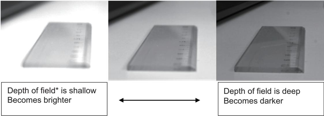
\*Depth of field: Depth at which focus is reached.
