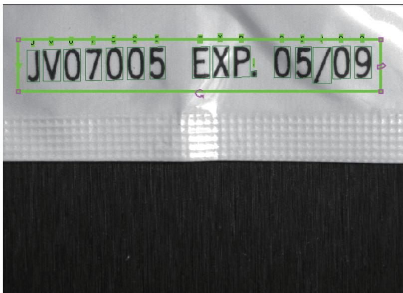
6. If the scanning fails for several times after the registration, adjust the region by the "Auto-Tune" function.
