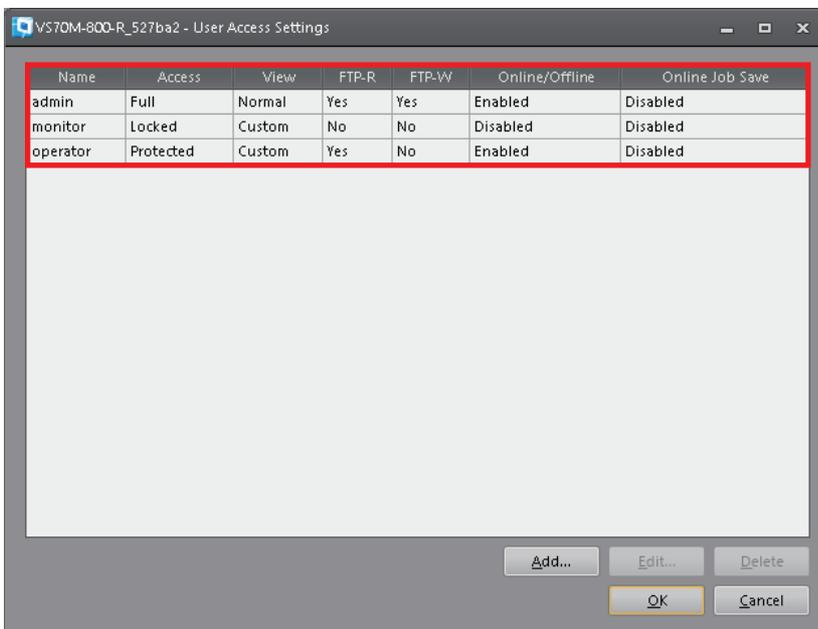
To switch users, click [Log On/Off] from the [System] menu in In-Sight Explorer to display the screen below. The logon user can be switched by entering a user name and password, and clicking Log On.
