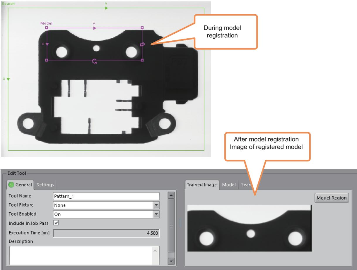
The "Edit Tool" screen has the following tabs: [General], [Settings], [Trained Image], [Model], and [Search]. Details of each item are listed in the Help section of EasyBuilder, which is described later.
