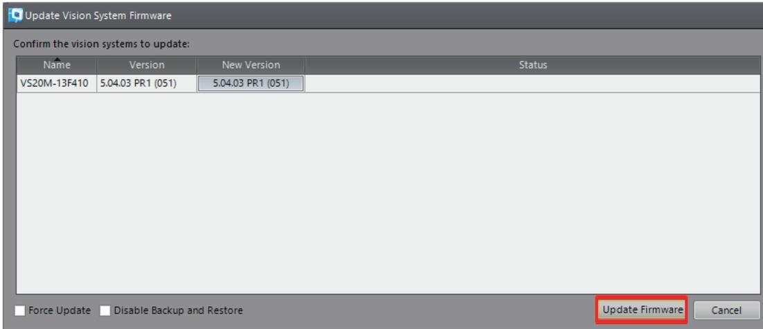
When In-Sight Explorer is connected to the corresponding vision sensor at this time, the following window appears, and the firmware update is stopped.
