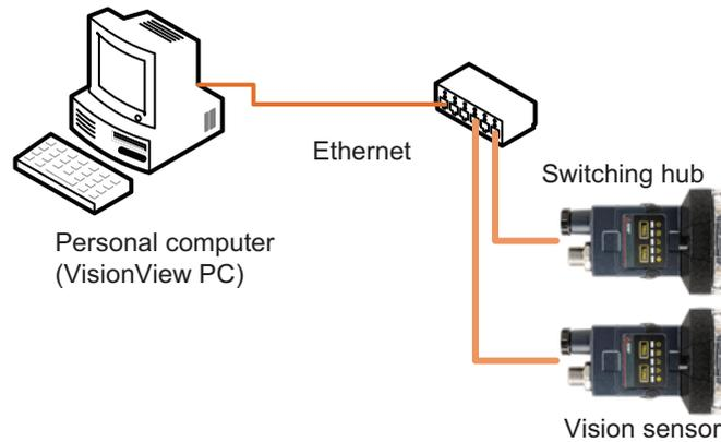
VisionView PC is software to realize the VisionView interface on the screen of a Windows personal computer. It is possible to monitor and adjust the vision sensor using the same interface as the VisionView 900 and VisionView VGA. A license is required for use.
