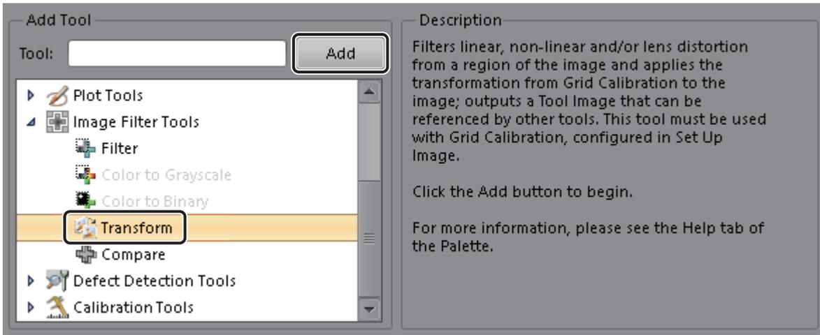
If [Transform] is added, and the region is configured, it is possible to check the image that was transformed according to the grid calibration results.
