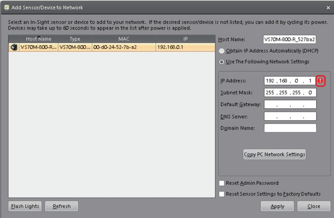
3. The warning mark disappears when an appropriate IP address is entered.
