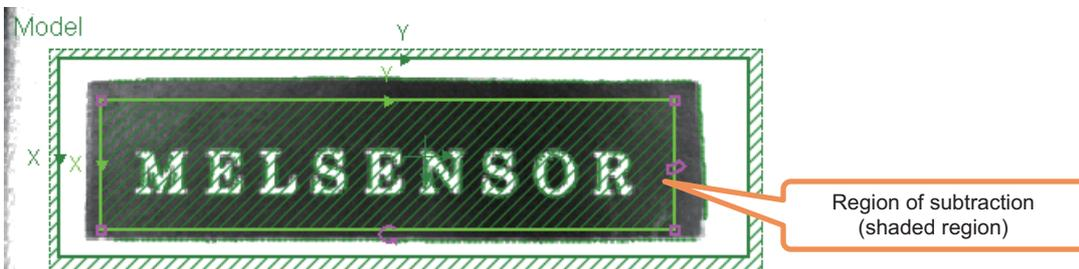
5. If [Train] is clicked at the [Model] tab, the section outside the subtraction region undergoes model registration again.
