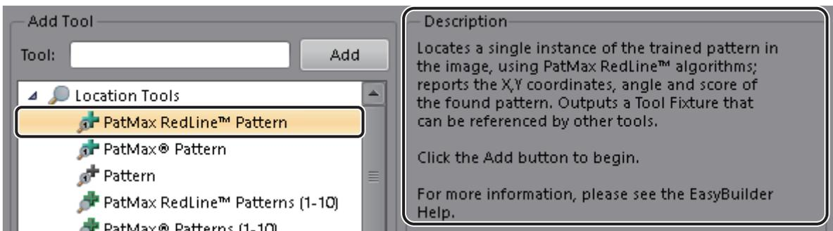
3. If the [Add] button is clicked, the tool is added to the job, and the display changes so that initial settings that comply with the added tool are configured.
