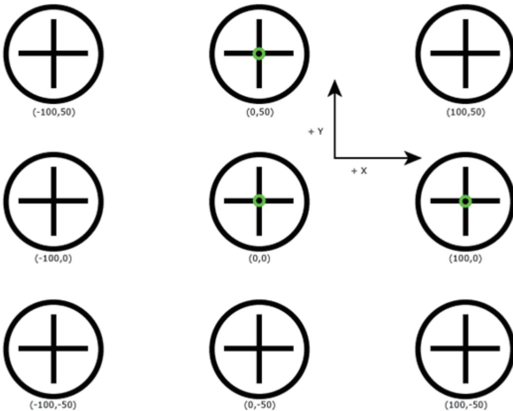
Before calibration, import a calibration plate image that includes nine targets arranged evenly spaced.
