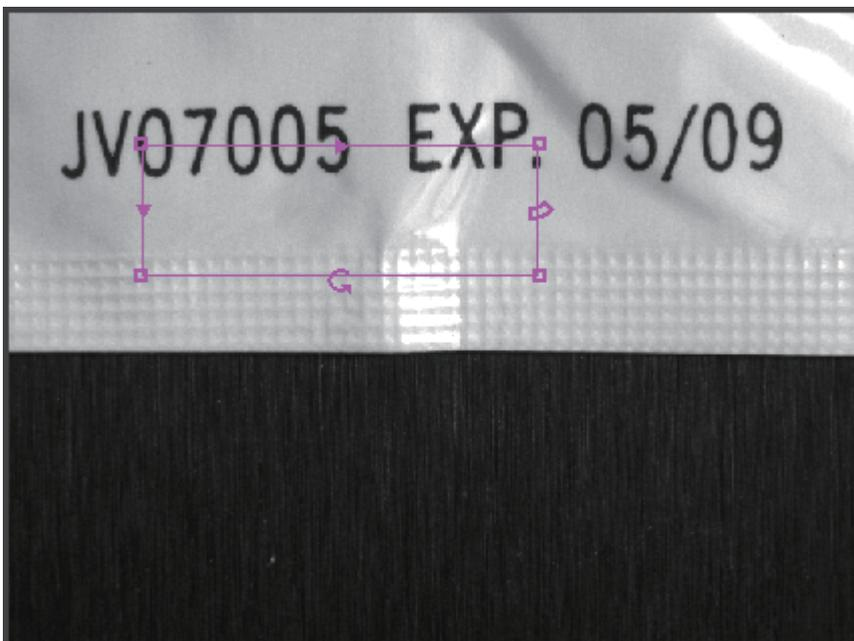
Configure the inspection region so it encloses the target text string to be read.
