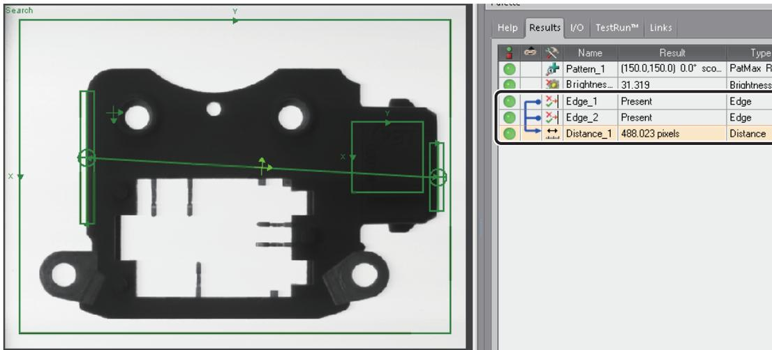
At the default value, distance measurement between edges is from center to center.
